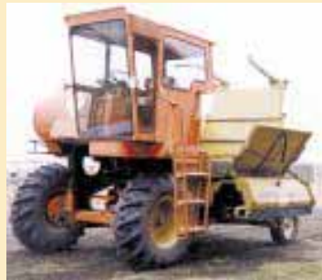
He removed the Haybuster's wheels and stripped everything but the cab and drive train from the combine. Then he attached the combine's rear wheels and steering axle to back of Haybuster frame.
