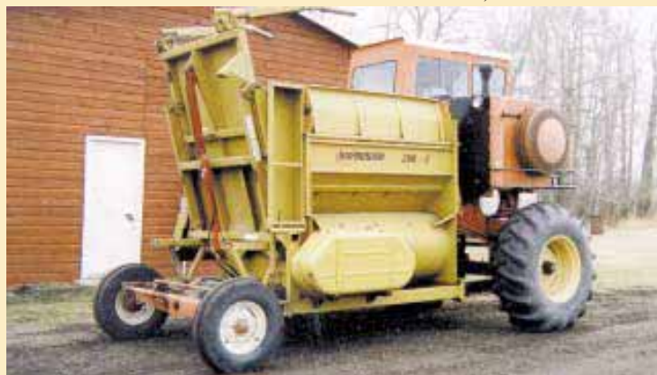
Unit distributes shredded hay for feed or spreads fluffy bedding.
