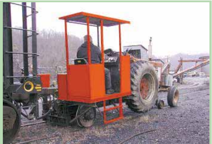
"Freightshaker" add-on locomotive turns any farm tractor into a mini locomotive that can be used in freight yards to move rail cars around.
