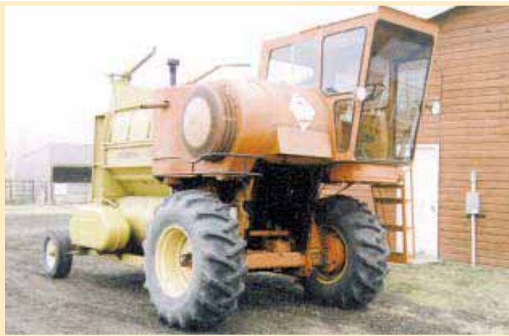
To make his Haybuster 256 big bale shredder more handy, Denis Brenneis mounted it on the frame of a Massey 410 combine.
