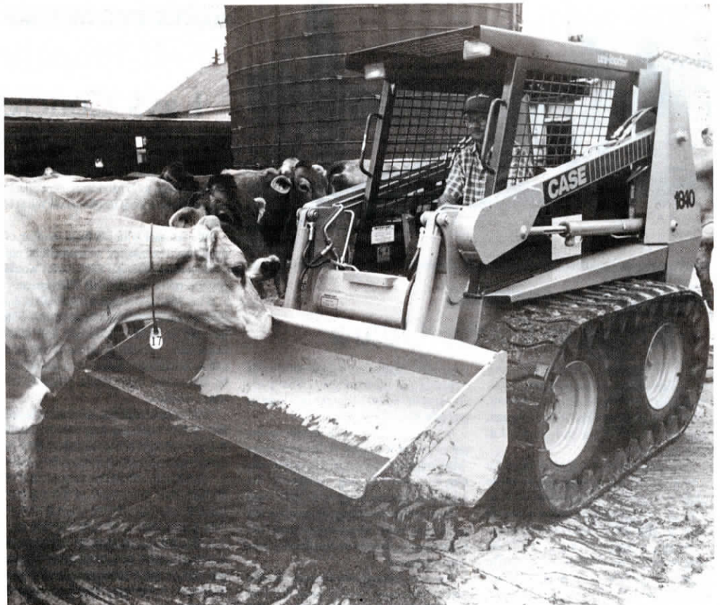
Goodyear has already started selling rubber tracks that mount on existing skid steer loaders. Tracks and specially-built undercarriages are being developed for most wheeled equipment, powered or not.
