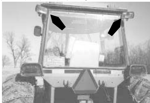
Two lights on back of cab replace original incandescent lights. Iager also added a yellow flashing marker light to each side of cab, as well as a strip of red and white reflective tape on back of it.
