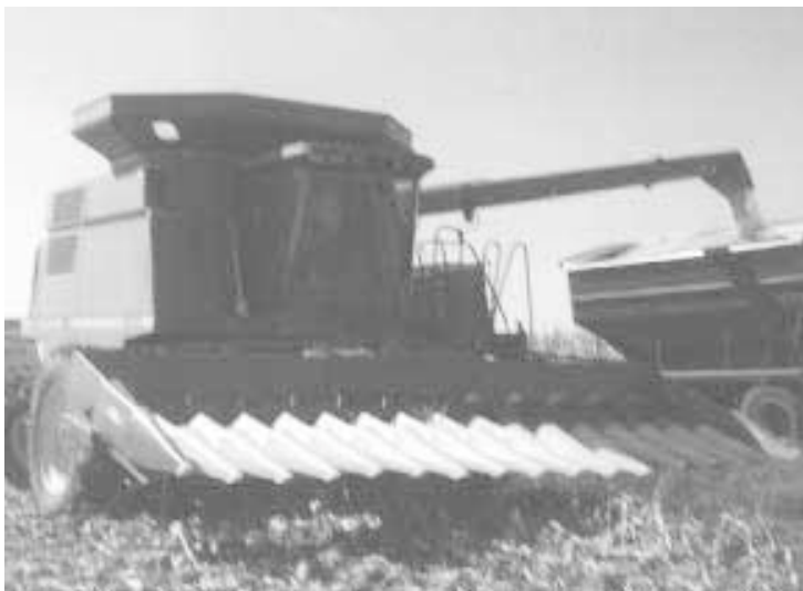
Rea's 6-row, 15-in. corn head has just one gathering chain per row. They built it using an 8-row Deere 843 head they already owned and bought two used 4-row heads.
