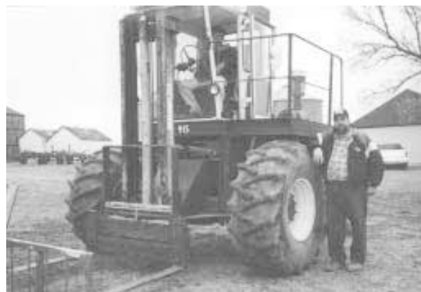
Roy Hawkins converted this old International 915 combine into a forklift. He uses it to lift heavy equipment onto shelves in his machine shed and for a variety of other jobs.
