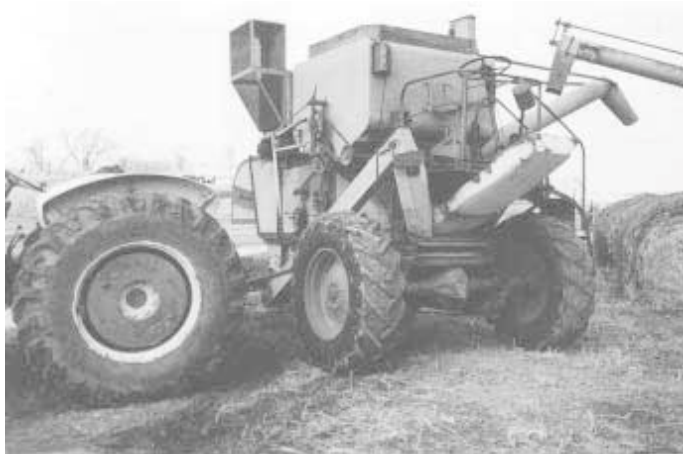
George Keener turned his old Baldwin combine into a high capacity, stationary grain cleaner.
