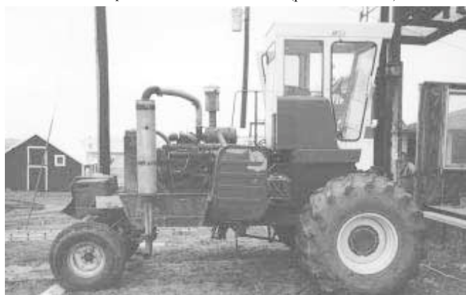
To counterbalance the load on front, Hawkins hangs 1,800 lbs. of tractor weights on back of frame. "I've lifted as much as 8,000 lbs. on the fork with no problems," he says.
