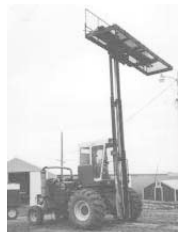
Lift raises 26 ft. high so Hawkins built a 4 by 16-ft. scaffold, with a 3-ft. high siderail to fit the fork, so he could use it to put new siding on his house.
