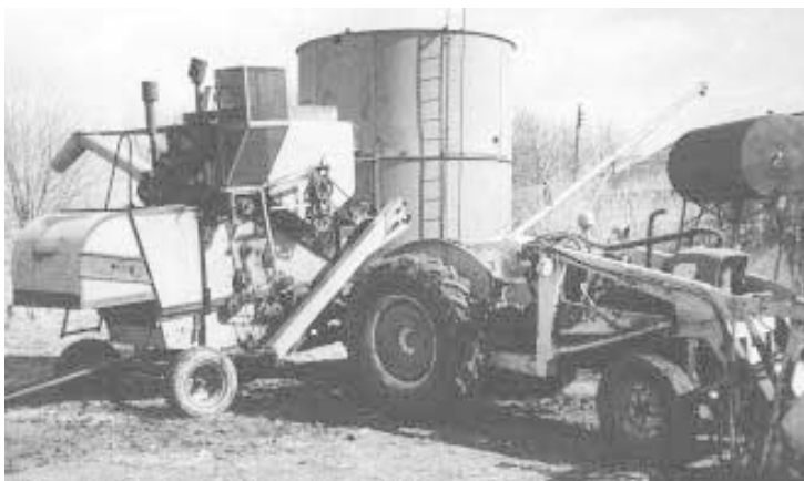
He removed the header and added a hopper to pour in the grain to be cleaned. Since the engine didn't run any more, he decided to power it with a tractor pto.
