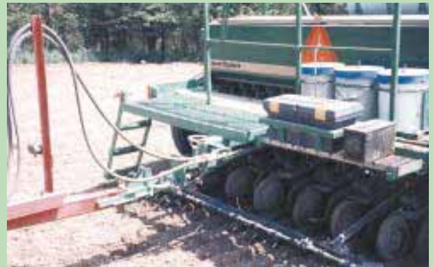
Pintle hitch allows packer wheels to swivel for flexibility when drill is raised to turn on headlands.
