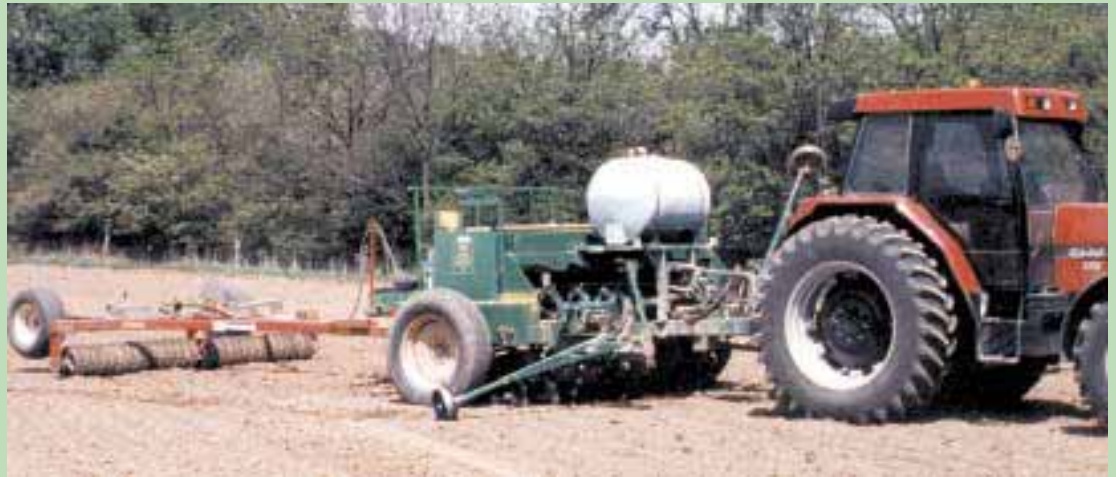
Mac Campbell and his son, Chris, put a hitch on back of their 10-ft. Great Plains drill so they can pull a set of packer wheels behind the drill to improve seed-to-soil contact and smooth out the seedbed.
