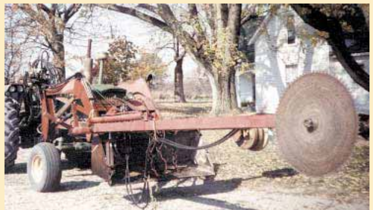
The 29-in. buzz saw blade is offset to side of loader which makes it easy to trim fence rows.
