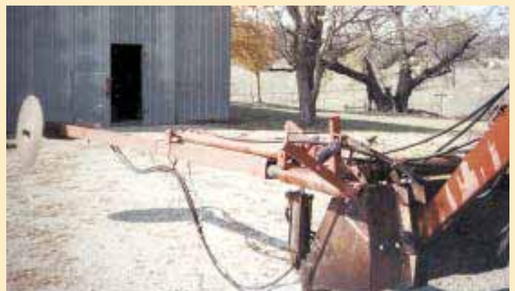
A 3 by 8-in. cylinder mounts on side of bucket to move buzz saw up and down. Altogether, about five different hydraulic movements can be made to change saw position.
