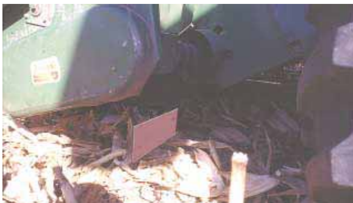
Steel plate (outlined in white in photo), bolts onto header frame positioned about 4 in. off ground. It simply bends stalks forward so they point away from tires.
