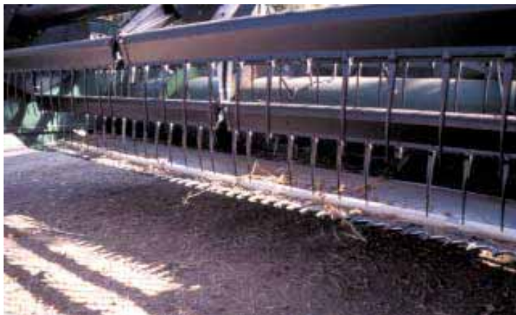
A length of 1 1/2-in. dia. PVC pipe clamps on about 8 in. behind the cutterbar.
