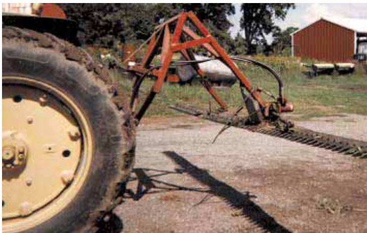
Hydraulic-operated, 18-ft. sicklebar works great for cutting off tall-growing weeds above Davis's edible bean crops two to three weeks before harvest.
