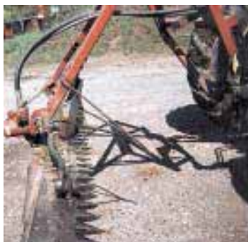
Knives are driven back and forth by a Gandy orbit motor.
