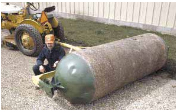
The 500-gal. LP tank is supported by axles at each end that came off a field cultivator.
