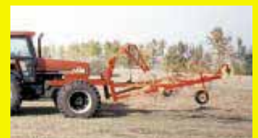
Each arm is suspended independently from a hinge point just in front of tractor.
