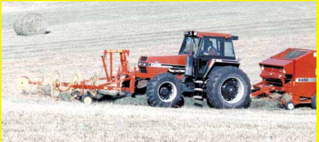
"There are many benefits to raking hay ahead of your tractor as you bale," says Henry Lutz, who came up with this 20-ft. wide front-mount rake. Six 36-in. dia. rake wheels mount on a steel frame that clamps to the loader arm brackets on any tractor.
