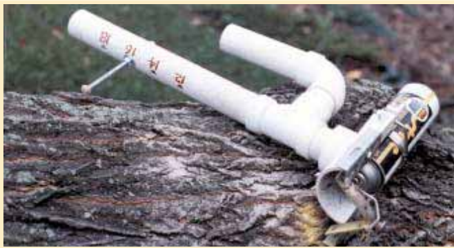
Firewood marker holds a can of yellow paint that's triggered by a "finger" that he bumps against log.
