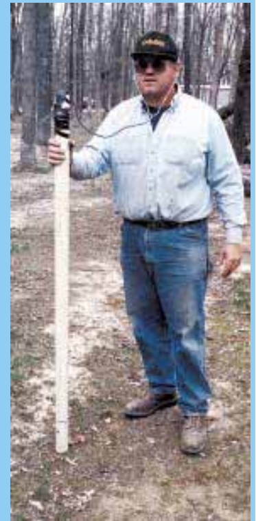
Himes taped a styrofoam cup upside down to the top of a 5-ft. long piece of 2-in. dia. pvc pipe. Then he taped a doctor's stethoscope to the bottom of cup.
