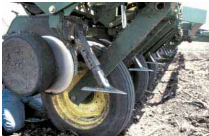
Shawn and Todd Flynn use ordinary 8-in. cultivator sweeps to clear a path ahead of the disc openers on their Deere 1770 planter.
