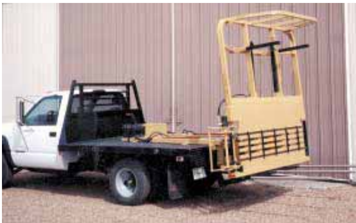
"My big bale flaker allows one person to both load and feed bales," says inventor Kenny Grellner. Unit mounts on any 8-ft. pickup flatbed.
