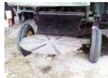
Trash from combine sieves falls down onto a 3 1/2-ft. dia. steel disc that's rotated by a small hydraulic motor. Rubber strips grab the material and help swing it off the disc.
