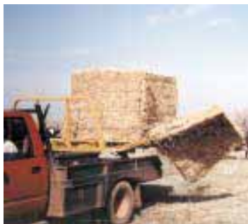
Rig uses a pair of motorized rotating forks to pull flakes of hay off bale.
