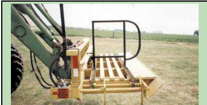
Grellner also makes a front-end loader-mounted model is also available. Note conveyor and push bar that are used to push bale off one side.
