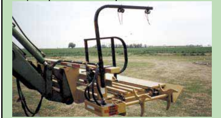
Grellner also makes a front-end loader-mounted model is also available. Note conveyor and push bar that are used to push bale off one side.
