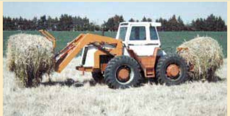
Reinhardt built a front-end loader for his Case 2670 4-WD tractor to carry two bales up front. A bale fork on the 3-pt. hitch holds two bales or more.
