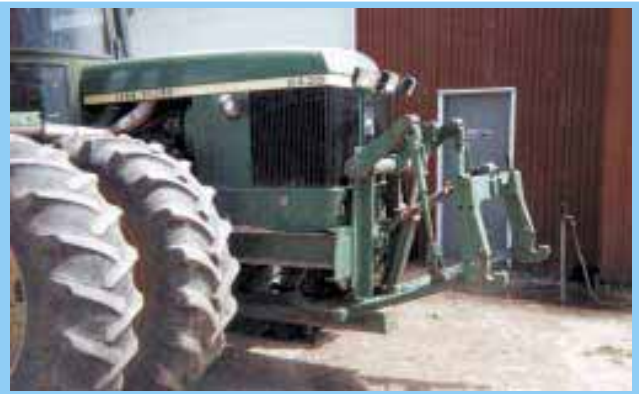
Home-built, front-mount 3-pt. hitch allows Robert Davis to cultivate and harvest edible beans with equipment that's out front and easy to see.
