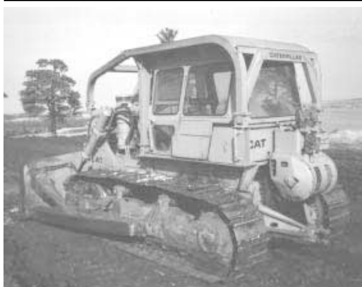
To add comfort to his D-7E Caterpillar, Steve Vogel of Yale, Iowa, added an old Hiniker cab to it. The cab had originally been mounted on a Deere 4520 tractor.
