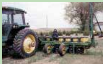
He mounted four gauge wheels on front of toolbar and two lift assist wheels behind it.
