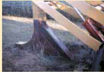
Tile plow is equipped with a 5-in. wide boot, with a blade on front that’s 3 in. wider to prevent “side dragging”.
