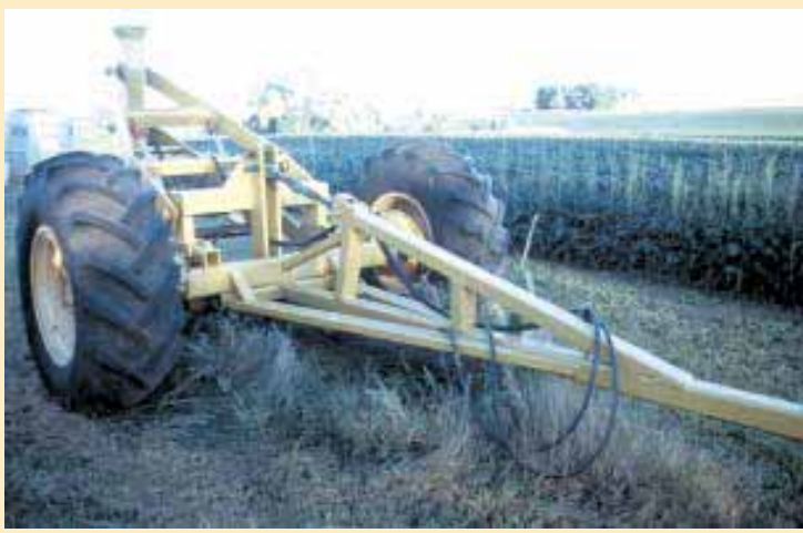
Kenny Brandt used the front wheels and axle off a Massey Ferguson combine to build his own “big wheeled”, pull-type tile plow.
