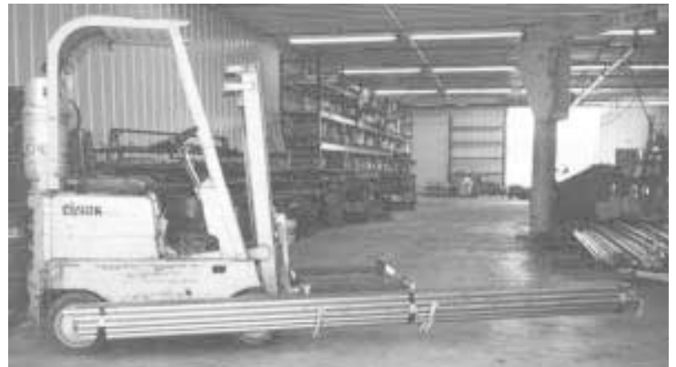
Side attachment carries load only a couple of inches off floor so there's far less chance of accidentally hitting something and dumping the load.
