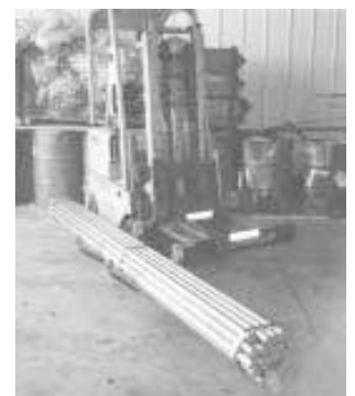
With the load carried alongside forklift, operator can get long stuff through narrow aisles and doorways.
