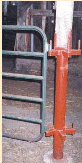
Gate hanger is designed so Kerr can lift gate off one set of hinges and replace it on one of two other sets, at a completely different angle.
