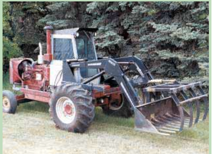
Stripped-down IH 815 combine is equipped with a quick-tach Leon front-end loader.
