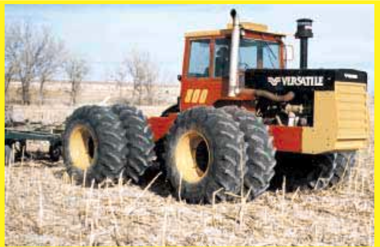
According to tractor rebuilder Harry Herl, Versatiles are relatively cheap to repair because many replacement parts can be bought from over-the-road truck parts shops.
