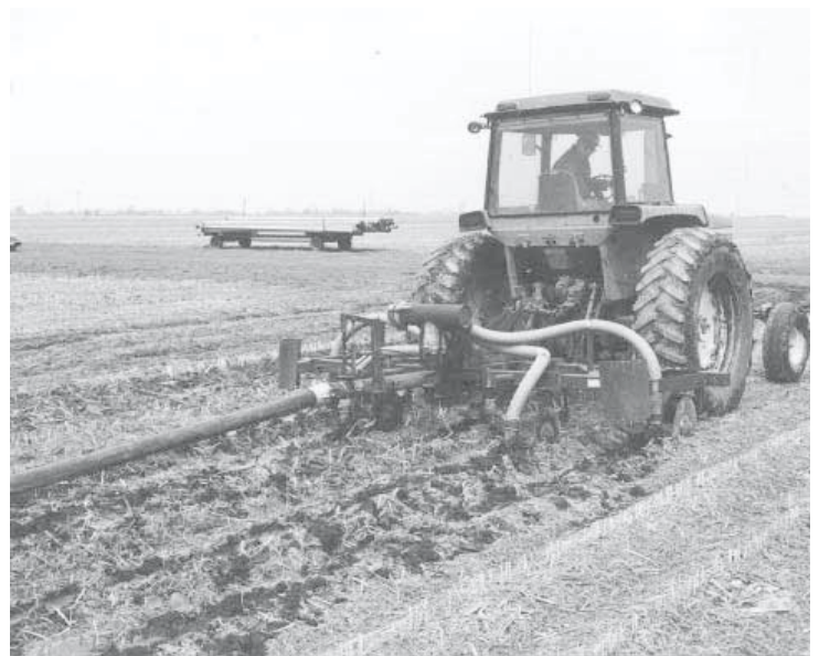
Tractor-mounted, 4-row injector is fed by a 660-ft. long, 4-in. dia. rubber drag hose that in turn hooks up to aluminum irrigation pipe.
