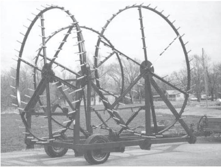
Rotary harrow has three non-powered rotating wheels, two in front and one in back. All three wheels fold up for transport.
