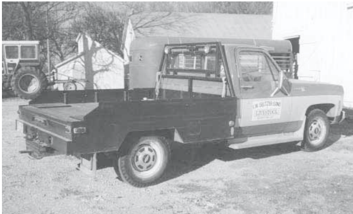
Seltzer replaced the rusted-out bed on his Chevy 3/4-ton pickup with a flatbed off a one and a half ton model that had been used as a portable welding rig.
