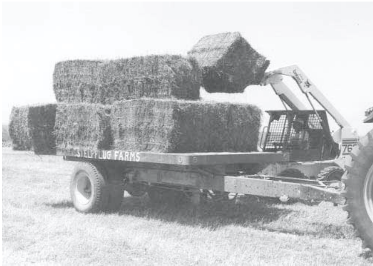
Gary Stelpflug converted a 1972 Ford F-600 2 1/2-ton truck into this pull-type flatbed. It holds up to 12 big square bales and dumps hydraulically for unloading.
