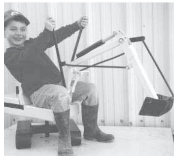
Linkage system on this toy excavator allows bucket to be controlled regardless of the position of the boom.
