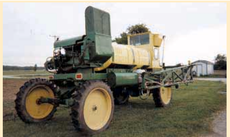
Sprayer rides on tall 12.2 by 38 tires. Combine still has the original air filtering system for the radiator (next to engine on back).
