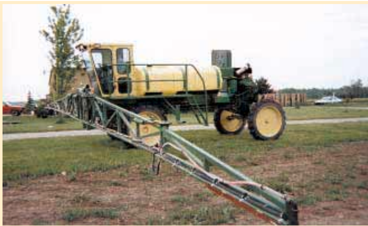
Deere 55 combines work great for converting into self-propelled sprayers, says Len Knipstein. With the help of a friend he built this sprayer equipped with a 60-ft. boom.
