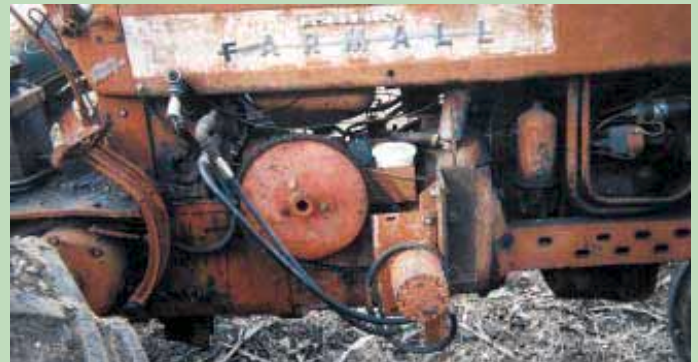
Davies modified his IH Farmall 450 tractor to get "creeper" speeds. He replaced the tractor's belt pulley with a large sprocket, which is chain-driven by a hydraulic motor.
