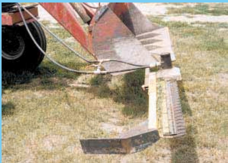
"It works great for mowing roadside ditches," says Myron Stadnick, who removed a cutterbar and orbit motor from his swather and mounted it on his front-end loader.
