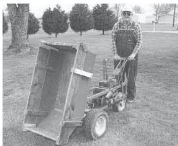
Dump box came off a commercial pull-type cart and dumps to the front.
