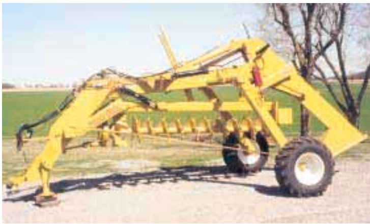
Trencher plow is equipped with a conventional boot as well as a 25-in. dia., 10-ft. long auger. The pto-powered auger can dig a trench up to 6 ft. deep in which tile is laid.
