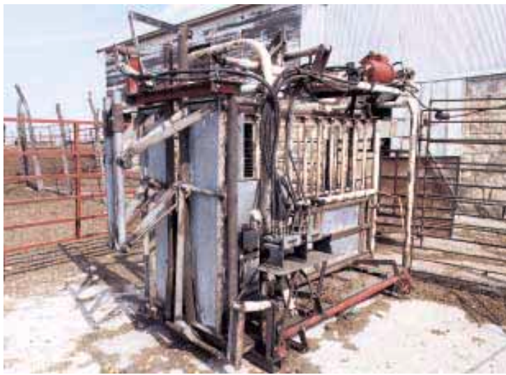
Using small hydraulic cylinders that he bought at an auction, Armin Scripser converted an old My-D Handy squeeze chute from manual to hydraulic operation.
