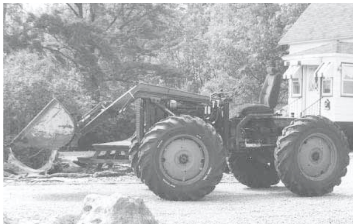
Linstad's 4-WD tractor is equipped with the rear ends off two junked WD Allis Chalmers tractors. It's powered by a Chevy 283 V-8 engine over the front axle. The bucket seat is from an old Chrysler car.
