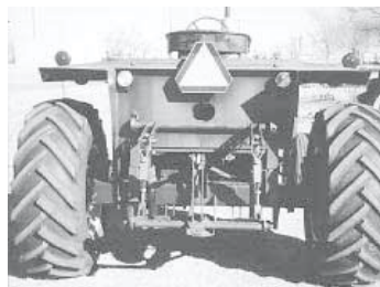
Valves for the 3-pt. hitch, as well as the 3-pt. lift cylinders, come from an IH 503 combine.
