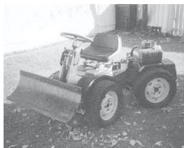
Pfannmuller's 4-WD utility tractor is only 32 in. wide and 69 in. long, but it's big enough to do all kinds of jobs.
