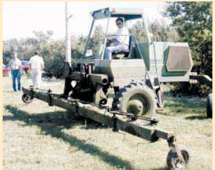
Home-built 23-ft. "weed whacker" mounts on front of Woolhouse's self-propelled swather.
