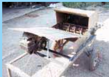
Chopper is big enough to accept a small square bale endways. Jason usually feeds in about a half bale at a time.
