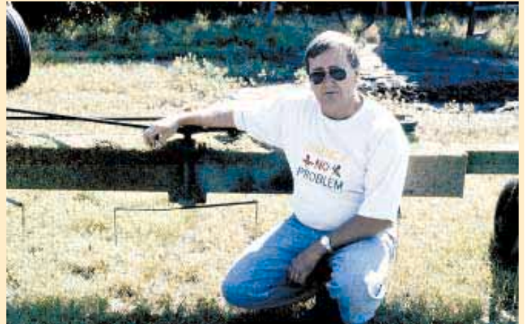
Woolhouse mounted nine rotating horizontal steel rods under the beam and hung a 6-in. length of chain from the end of each strap. Each "blade" is fitted with a pulley that's belt-driven off the swather driveshaft.
