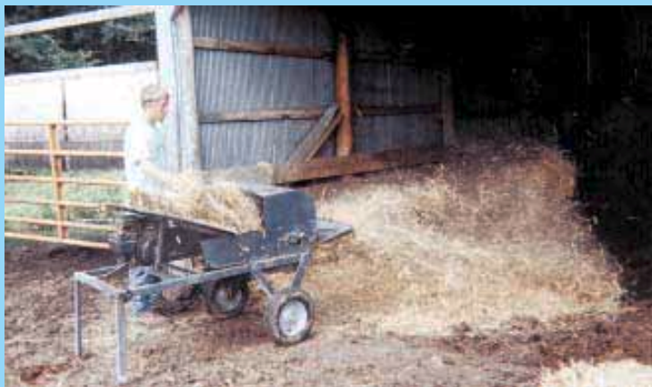
Straw chopper is powered by a 5 hp Briggs & Stratton gas engine and can be wheeled anywhere.
