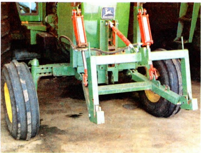
Hass built the hitch to carry ridge-shaving units while pulling rear-mounted planter.
