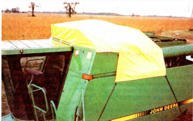
Custom-fitted tarps, made from 18-oz. coated vinyl, can be left in place while combining or rolled back out of the way.
