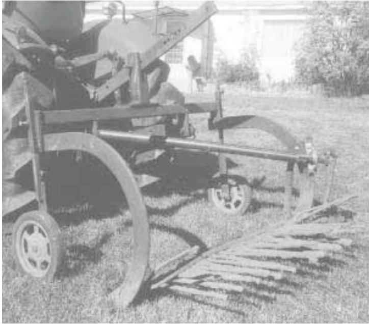
The 3-ft. wide digger is equipped with a series of 16-in. long steel tines spaced about 2 in. apart. A pair of small rubber wheels mount ahead of tines to control their depth.
