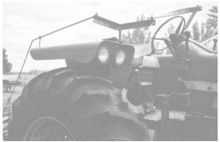
Linkage consists of two long steel rods. One hooks up to the pto control lever and the other (above) hooks up to the throttle.
