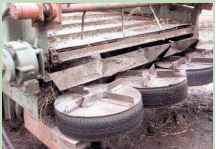
A flat plate bolts to top side of each wheel rim. Four pieces of 3-in. angle iron are welded to each plate to form paddles.
