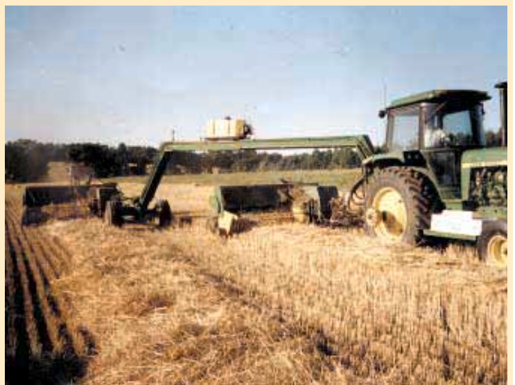
Hainsworth uses his hydraulic-powered hitch to pull two Deere small square balers behind his Deere 4440 2-WD tractor.
