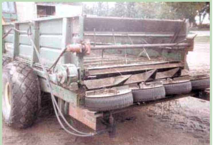
Soda mounted a row of four tires across back of box to act as spinner-spreaders.
