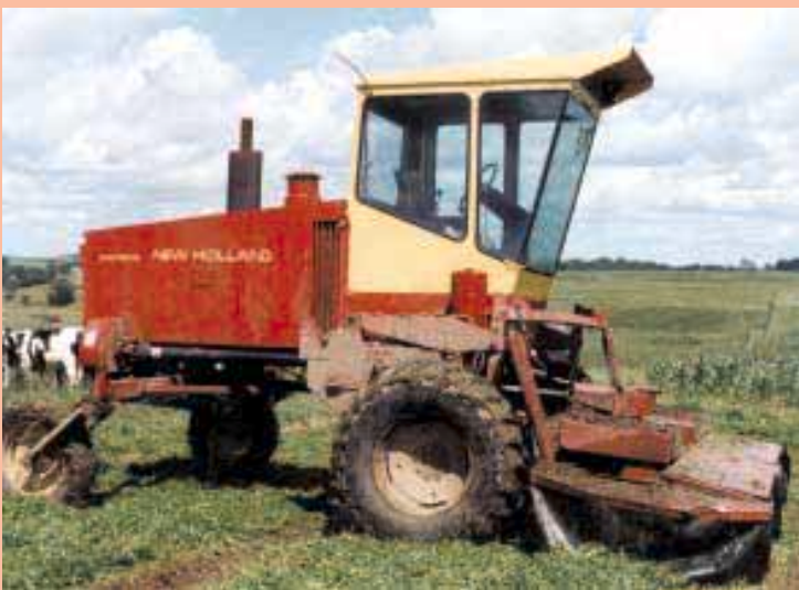
To build his self-propelled rotary mower, Balmer mounted the header from a pull-type 12-ft. Hesston Hydra-Swing Discbine on a Hew Holland sicklebar Haybine.
