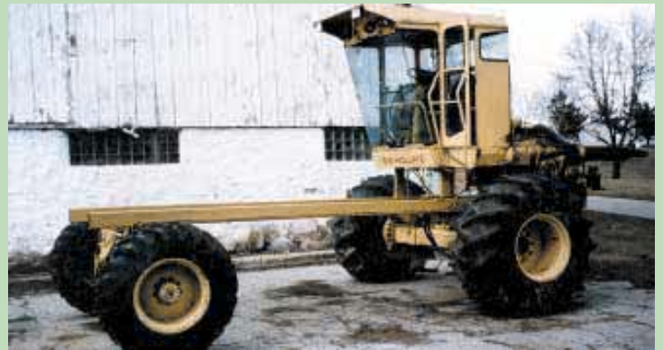
To build their 4-WD sprayer, the Sodas started with a New Holland 75 combine.
