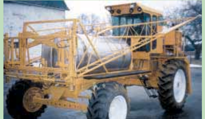
Sprayer is fitted with a 1,000-gal. stainless steel tank and 60-ft. boom.
