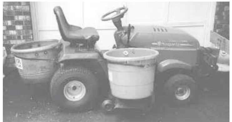
To pick up litter along highways, Vernon Feiler of Ocala, Fla., straps a pair of 25-gal. plastic tubs to his Husqvarna riding mower.
