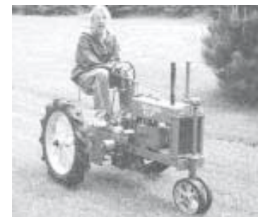
Ken Java's half-scale 1936 Deere B looks and works just like the real thing. He built it mostly from junk.
