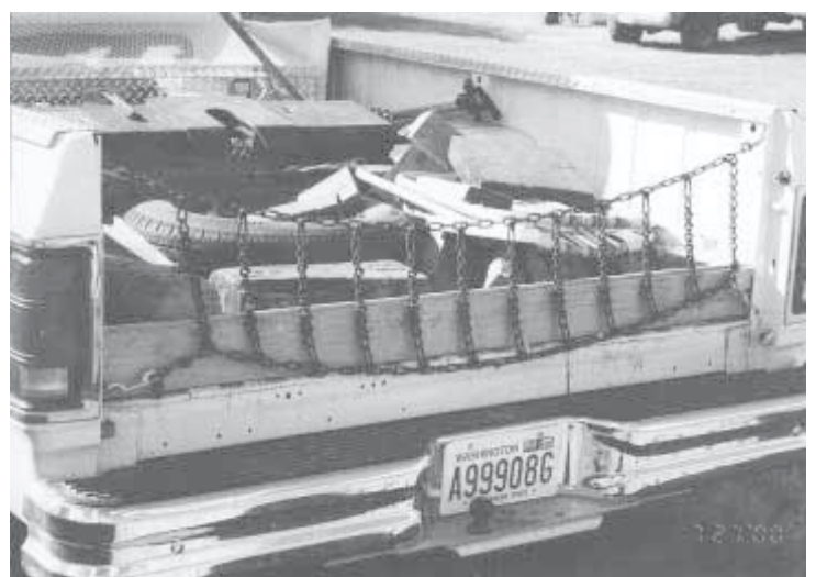
"Ordinary car tire chains can be used to make handy, fuel efficient tailgates for pickups," says William Erickson, who used the idea on his 1992 Dodge pickup.
