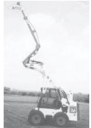
Crane is built in three sections. Lift capacity ranges from 1,500 lbs. when retracted, to 500 lbs. at full extension.
