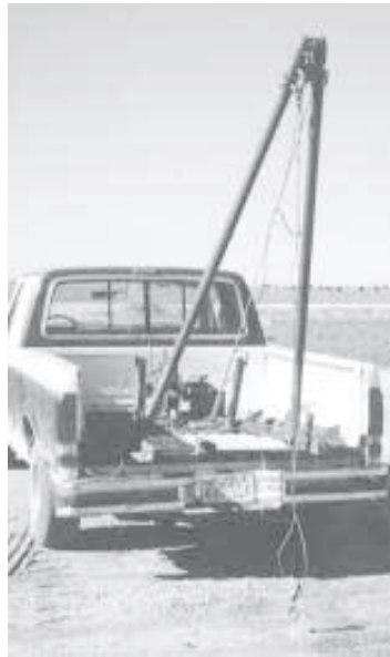
Winch attaches to pickup's gooseneck hitch and consists of a steel frame that supports a pair of gin poles.
