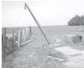
When not in use, Lamb stores winch by hooking it to fence post so it's standing up, ready to slide into pickup bed.
