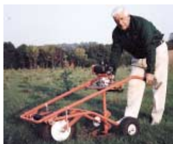
Cart-mounted auger drills 19 in. deep.
