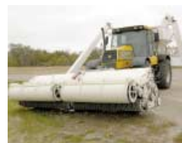
Paddle conveyor carries grain back to trailing wagon. Straw is left standing in the field.
