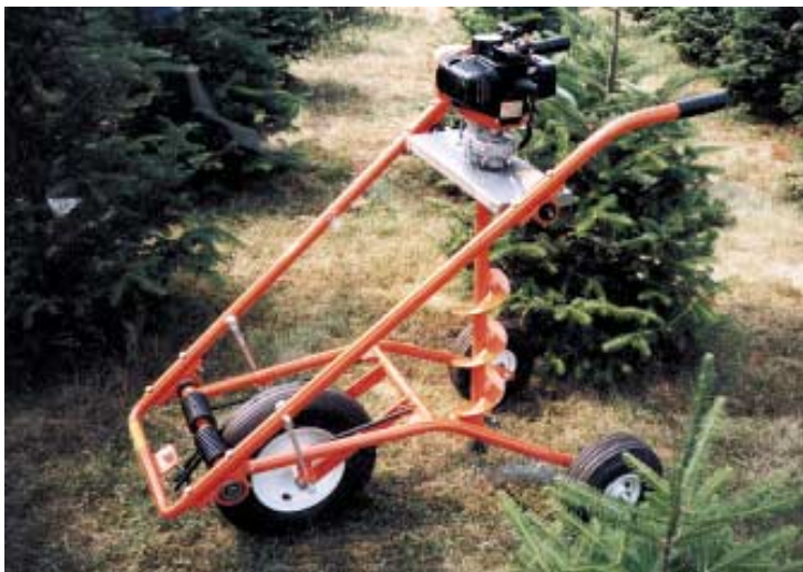
Cart lets one person do the work of two. Wishbone-shaped frame pivots up and down, controlled by heavy springs that hold the auger up unless you push down.
