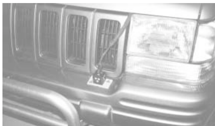
Plastic device attaches to vehicle's front bumper and has plug-in access on five sides.
