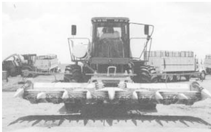
They use 8-row Austrian-built Kemper headers on the choppers. Power is supplied by new 600 hp 3456 Caterpillar diesel engines.
