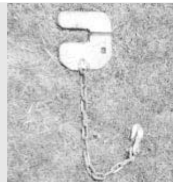
Slotted steel plate is attached to a 2-ft. length of chain with a hook on the end.
