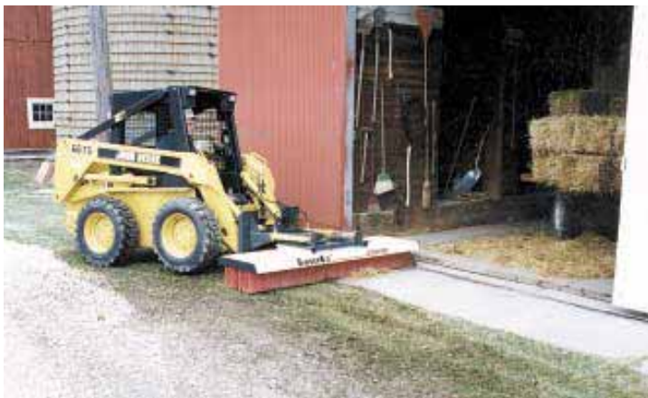
The "SweepEx" can be mounted on a skid loader and used to remove debris anywhere.
