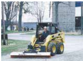
Unit's 12-in. long, replaceable poly brushes are tough enough to withstand use on gravel driveways.
