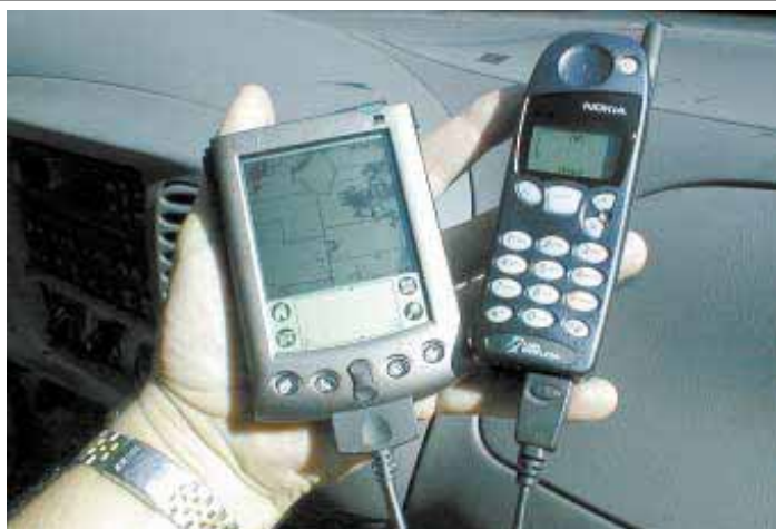
Service uses a Palm hand-held computer and a data capable cell phone. They're installed using a cradle that can be installed in any machine equipped with a cab.
