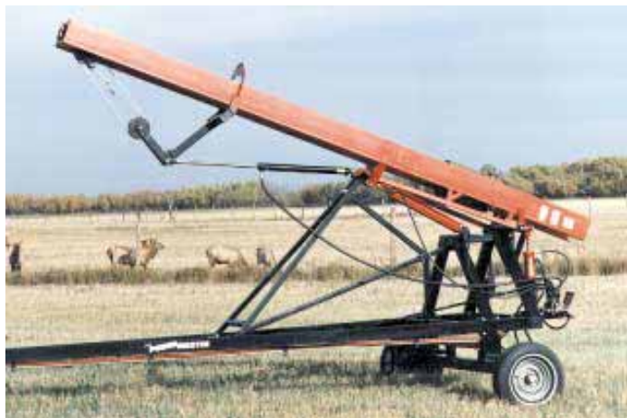
Trailer-mounted unit has a 1,000-lb. hammer that's raised by a long hydraulic cylinder. A separate cylinder is used to tilt the mast forward at an angle for transport.
