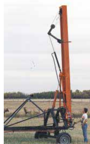
Hydraulic cylinder attaches to a steel cable which raises the hammer. Hammer free-falls onto the post once it reaches the top.
