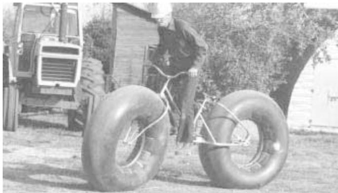
"Bug Squasher" uses 24 by 12-in. tractor tire inner tubes fitted to the rims of a 26-in. bicycle frame. "An experienced rider can mash a lot of hoppers with it," jokes Jaegli.
