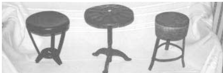
Stool at center was made with the lid off a corn planter. Metal stool at far right uses a milk can lid for the seat.
