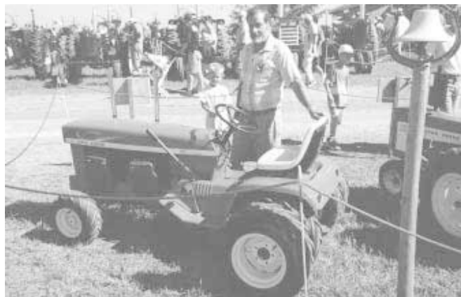
Pat Prom made this "double engine" Deere 110 garden tractor by stretching it out 15 1/2 in. and adding a second engine.
