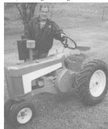
Prom built this half-scale Deere 730 from scratch. It's powered by an 8 hp Kohler gas engine that belt-drives a Peerless transaxle.
