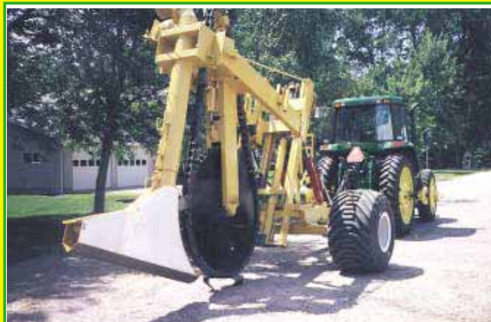
Tiler’s digging chain wraps around 6-ft. dia. wheel and a pto-sprocket on top of the machine. V-shaped cutting teeth rotate toward the tractor.
