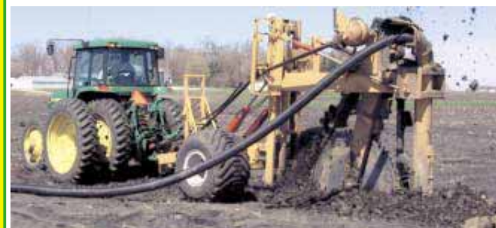
Tractor is fitted with “creeper” gears to run slow enough for tiler to cut a slot for plow shoe. It can be operated by a 170 hp. tractor, much smaller than other tilers.
