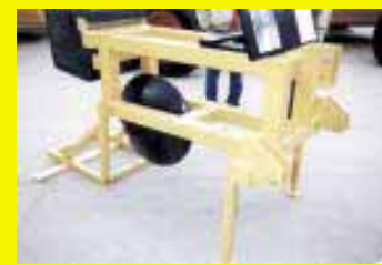
Ditcher consists simply of a pair of disc blades welded together face-to-face and mounted on a 3-pt. frame.
