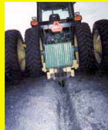
Tractor weights mount above ditcher wheel to keep it in the ground.
