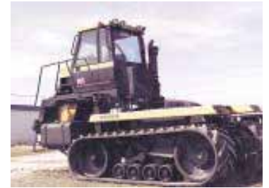
Scheetz stripped the Cat Challenger down to the frame. Then he remounted the cab further ahead on the frame, raising it 16 in. and reshaping the hood. He also eliminated the back fuel tank and fitted the tractor with saddle tanks. He installed a first-of-its-kind sliding fifth wheel hitch on back of the Challenger frame to pull the planter, which is fitted with a detachable "gooseneck".
