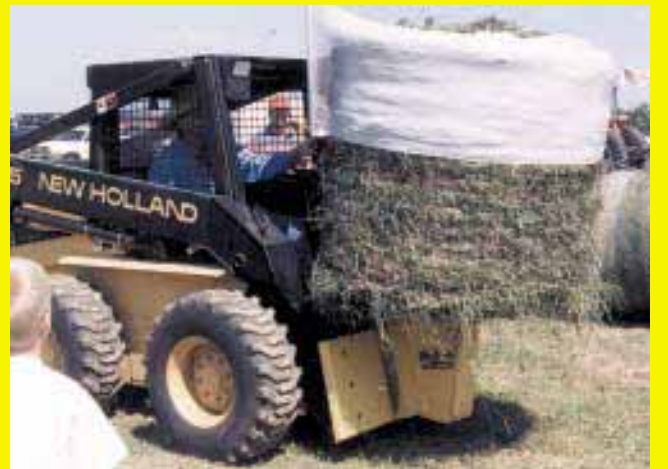
To wrap a bale the operator spears it and tips it up almost 90 degrees. Then he rotates bale to wrap the plastic around it and uses the loader to raise bale at the same time.
