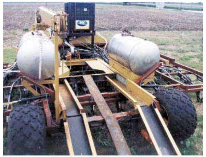
A winch pulls a 1,500-gal. anhydrous wagon up ramps and onto the planter, next to a pair of water tanks. Boom lifts bulk seed container into place.
