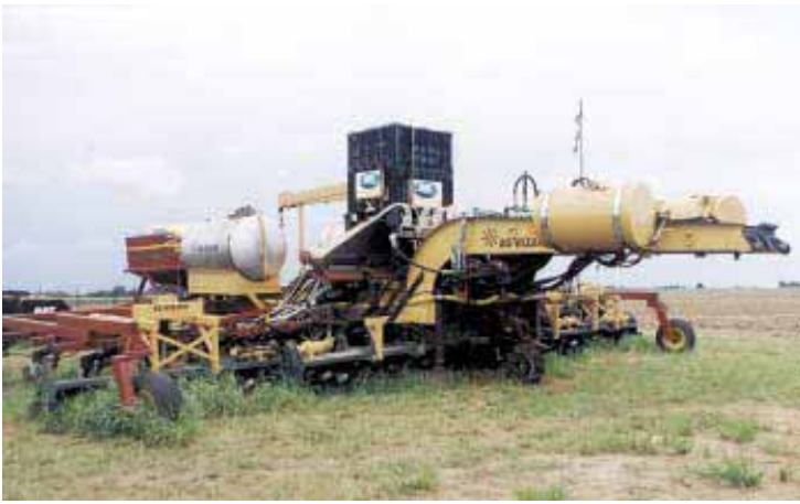
Scheetz welded a semi trailer fifth wheel hitch onto the frame of a Seed Hawk planter. The hitch carries all the weight of the planter.
