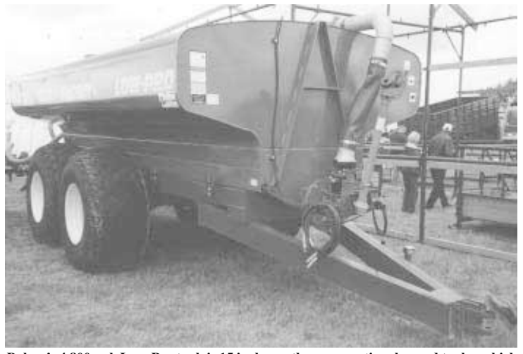
Balzer's 4,800-gal. Low-Pro tank is 15 in. lower than conventional round tanks, which allows you to see the tank's fill port from the tractor cab. That makes the tank easier to load and also lowers the center of gravity for better stability.
