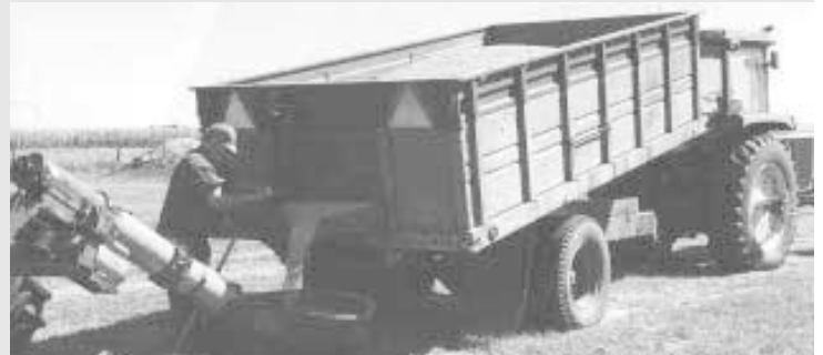
Becker removed the cab and engine from a 3-ton grain truck to build this grain wagon.
