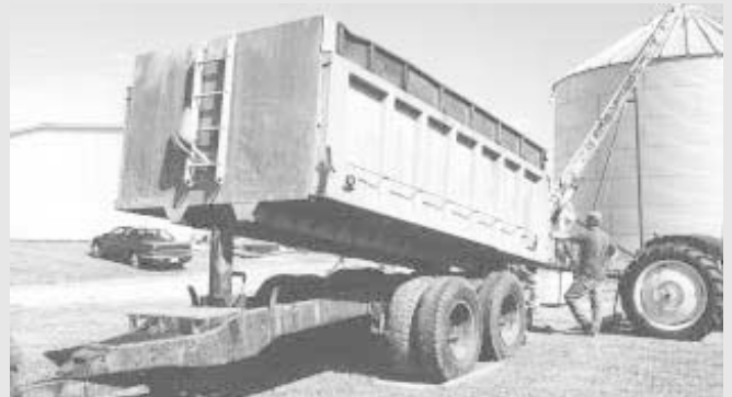
Stier used the running gear from a tandem axle truck to make this 500-bu. dumping grain hauler.
