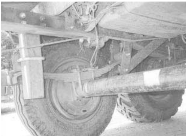
Jones removed pickup's rear bumper and bolted on a pair of 4-in. angle irons which extend the pickup frame by 18 in. A vertical length of 4-in. sq. tubing is U-bolted to each angle iron and also clamped to the back end of each spring on the extra axle.
