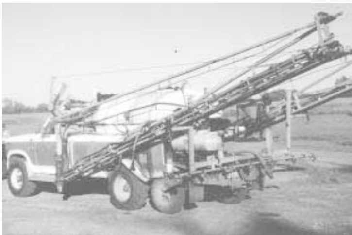
Jones mounted the wheels, axle, and springs off a trailer house on back of his 1985 Ford F-350 1-ton pickup. It's equipped with an 88-ft. spray boom.
