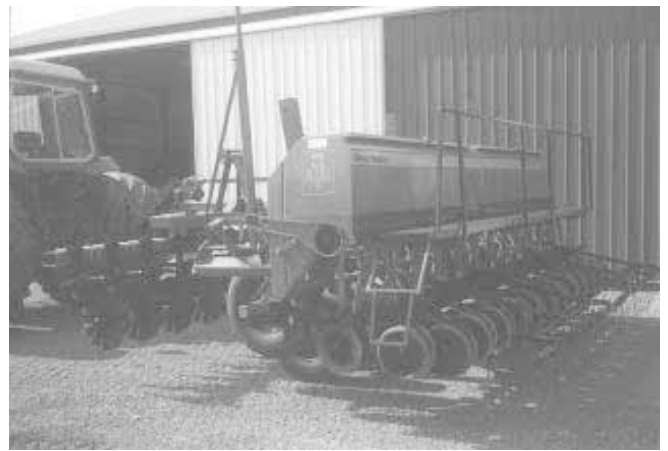
Ralph Brinkman made this 32-in. high “safety railing” for his Great Plains no-till drill to make filling seed hoppers safer.
