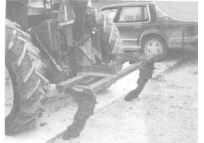
Subsoiler is made from a pair of old Deere moldboard breakaway plow beams spaced 5 ft. apart. Moore pulls rig behind his Deere 2-WD, 50 hp tractor.
