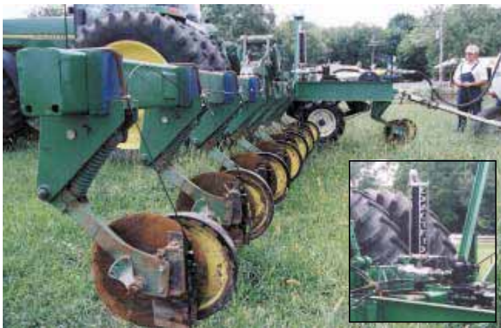
Allan Owings, Kansas City, Mo., applies anhydrous with toolbar-mounted single disc openers at speeds up to 12 mph, thanks to the Exactrix system, which puts 100 percent of NH 3 into the ground as a liquid. Owings places it in bands 4 in. deep.
