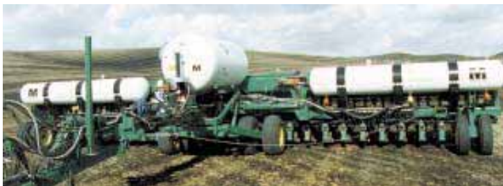
Steve Wilson farms 5,000 acres near Colfax, Wash. He mounted an Exactrix system on his Deere 455 no-till drill to apply anhydrous in 15-in. bands as he seeds winter wheat. He says the accuracy of the liquid system, plus the minimal soil disturbance from using disc openers, is what makes the practice possible. He averages 6 1/2 mph while seeding and applying NH 3 at the same time.
