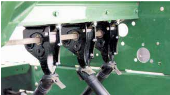
New Belt Meter units mount around drill's existing drive shaft. What makes them unique is the way they handle different size seeds. For example, if you set the drill to plant two beans per foot, they will hold that spacing regardless of seed size.
