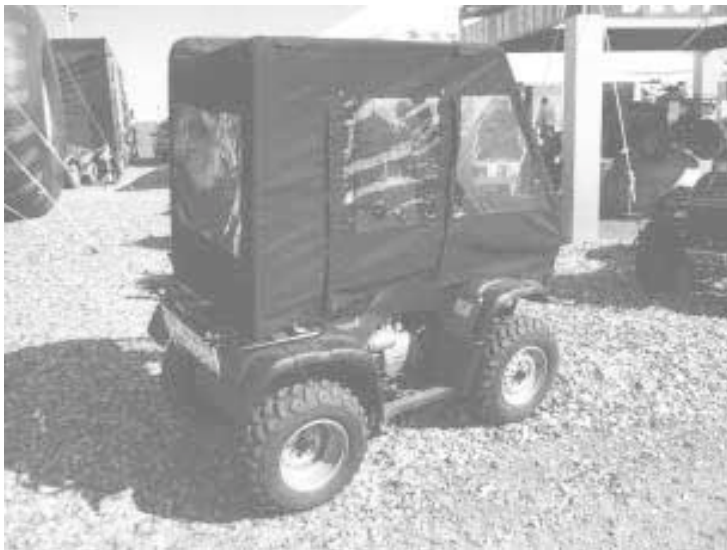
Wind and waterproof enclosure is made from heavy-duty poly stretched over a strong but lightweight steel frame that attaches to front and rear brackets on ATV.
