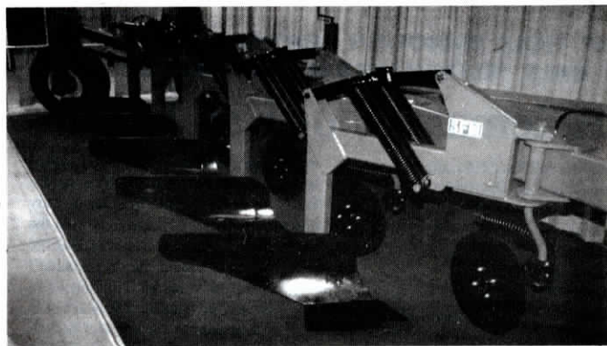
Long, slim moldboard bottoms turn soil part way over leaving 20% of residue on top.
