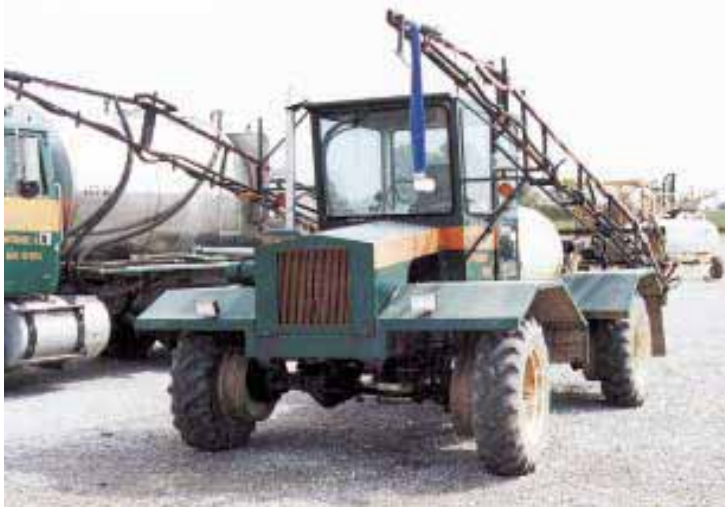
Home-built, self-propelled sprayer is equipped with “spacer wheels” for post emergence spraying in 30-in. corn and beans.
