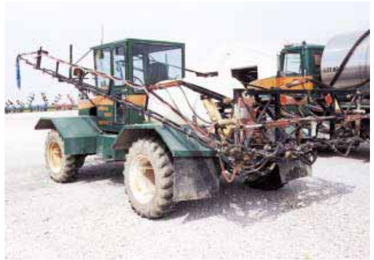
Sprayer is equipped with a 250-gal. tank and 45-ft. boom.
