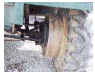
To make the offset “spacer wheels”, the Elliotts welded steel plates onto both ends of 12-in. wide steel drums and then welded the drums to the hubs of each wheel.
