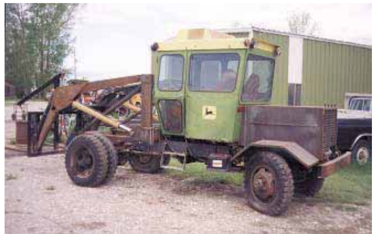
Forseth converted a 1 1/2-ton 4-WD military truck into this low-cost loader tractor. Loader is home-built while the cab is off a Deere 7520 4-WD tractor.
