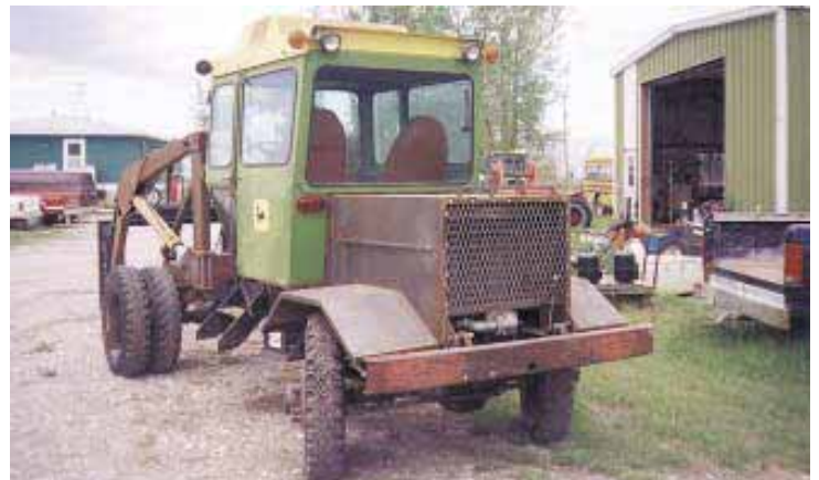
Rig is powered by a Chevy 6-cyl. engine on back that’s covered by a tilt-up hood.
