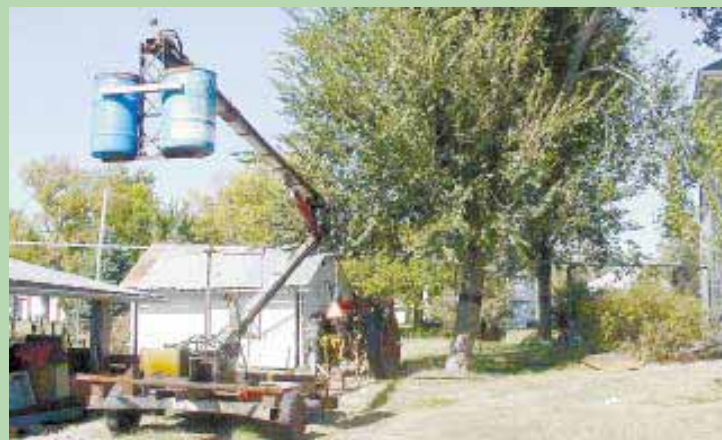
Pinkerton's home-built cherry picker goes up 40 ft. and swivels 45° to either side. It's powered by an 8-hp. gas engine with a 5-gal. hydraulic pump.
