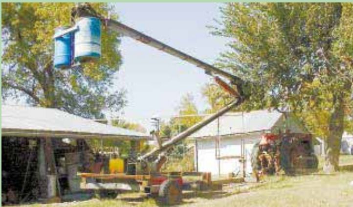
Pinkerton's home-built cherry picker goes up 40 ft. and swivels 45° to either side. It's powered by an 8-hp. gas engine with a 5-gal. hydraulic pump.
