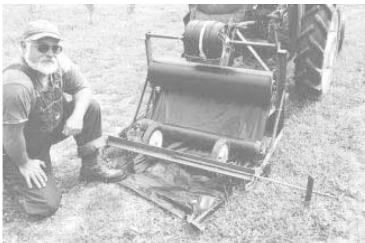
Dunn’s machine shapes planting beds, lays down drip irrigation hose, and then covers seedbed and drip hose with a 3-ft. wide layer of black plastic.
