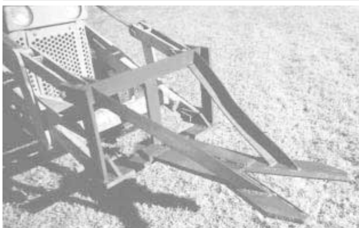
V-shaped pusher has a 3/4-in. steel bar that’s welded to inside edge of “V”. It provides a good grip on tree trunk without cutting it off.
