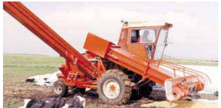
Rotating conveyor uses a swivel taken from a utility company's bucket truck. Machine loads semi-trailers in minutes without the operator so much as touching a shovel.
