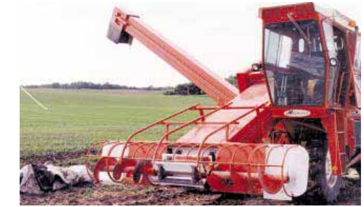
To make the SP grain loader, Brandenburg mounted an auger and a pair of conveyors on the frame of a hydrostatic-driven Uni-Harvester.
