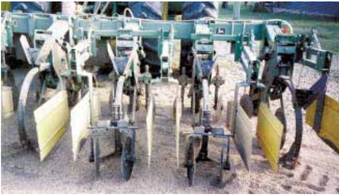
Covering discs mount behind the sweeps on Heitmann's Deere 885 cultivator. Discs throw soil back over the slit left by the sweep, so the soil doesn't dry as fast.
