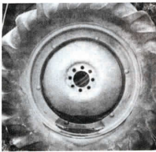
Horton removed the center hub on Ford wheel (left) and welded it inside combine wheel (right).
